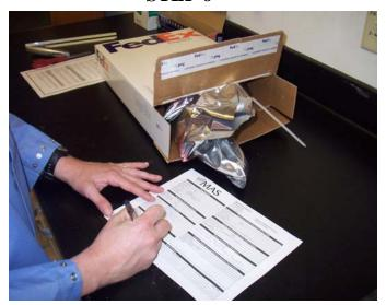
Place Mylar bag (containing samples) in sturdy cardboard box along with completed chain-of-custody form and send to:
