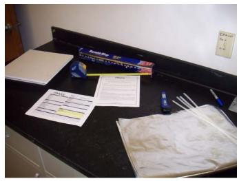
Assemble necessary supplies aluminum foil, chain-of-custody (COC) form, zip ties, ruler or tape measure and cutting device (scissors snips or knife)
