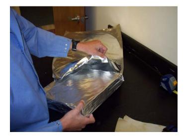
Following collection/cutting of samples, <u>immediately</u> wrap the stacked sample squares in 2 layers of **aluminum foil** and place in supplied **Mylar** sample submission bag.
