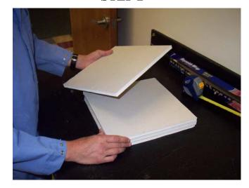
Select flooring samples from production line (if none available, obtain samples from post production stacks or consumer/retail sales packages). Select flooring at least three tiles or planks down from the top of the stack/package. Place **four** (4) selected samples face to back on top of each other to form a stack for packaging.
