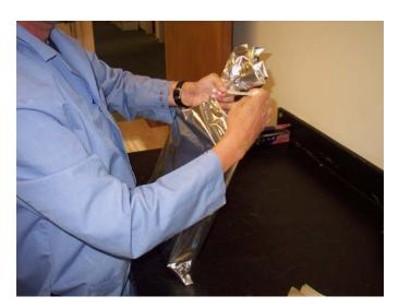
Squeeze all excess air out of Mylar bag and twist "open" end of bag tightly several times to close.
